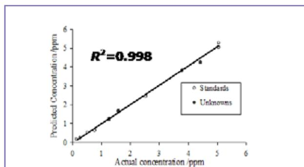
**Figure 3: Linear calibration graph of nicotine concentration derived from peak intensities shown in Figure 2.**
