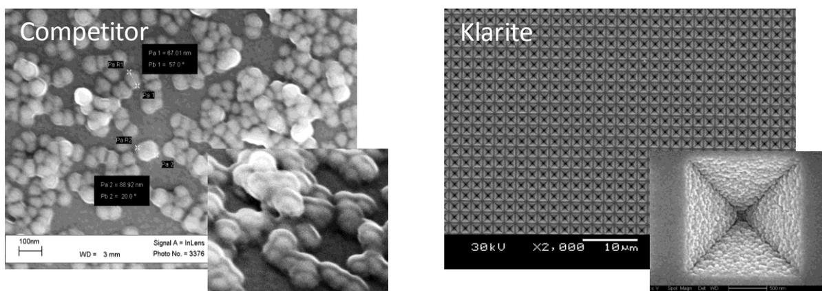
Figure 1 – SEM micrographs showing the surface structure of the two silicon-based substrates. Note that scale bars used are different (LHS - 100 nm, RHS - 10 $\mu\text{m}$ ) in order to properly compare features of interest.
